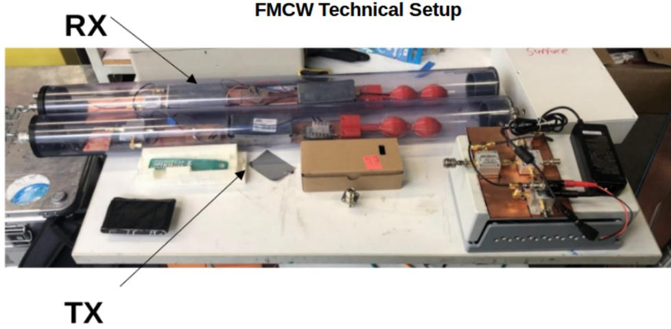
Figure 6.6: All of the components of the permittivity radar, except for the long coaxial cables, shown together on a table. The transmitter (TX) and receiver (RX) are shown, housed inside transparent PVC tubes (in the end, grey PVC tubes were used on the field). On the bottom right is the ‘controller’ board, which consists of a splitter and BiasTees to send the reference signal and power to RX and TX via cables.
