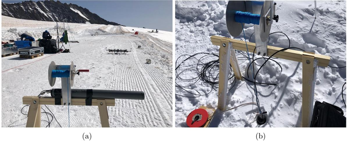
Figure 7.4: Calibration air-air measurements between TX and RX at the Test Site 7.4a, taken before the boreholes had been prepared. The photo is taken at L1. The RX tube is shown in the foreground, and is taped to the wooden stand. 42 m away is the TX tube at the location of L3. Deployment of the RX in to the L1 borehole (7.4b)
