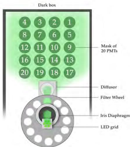
**Figure 4.5.:** Draft of front view of optical path with LED grid, iris diaphragm, filter wheel, diffusor and PMT mask.
