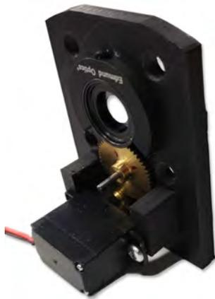
**Figure 4.17.:** Iris device with diaphragm driven by gear wheel connected to stepping motor [35].
