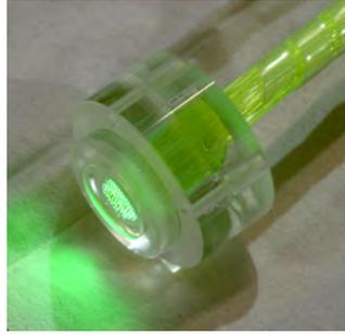
**Figure 2.13.:** Picture of optical connection from the WLS to the PMT, called a "Cookie", from [25, p. 24].
