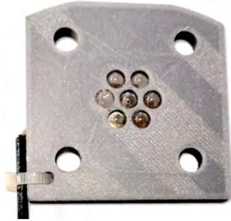
**Figure 4.9.:** Picture of the grid comprising seven single LEDs [35].
