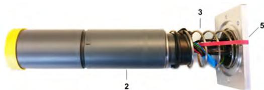
**Figure 3.9.:** Fully assembled PMT unit.
