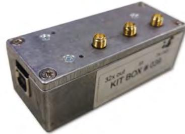
**Figure 4.31.:** Picture of the attenuation/amplification prototype from KIT.
