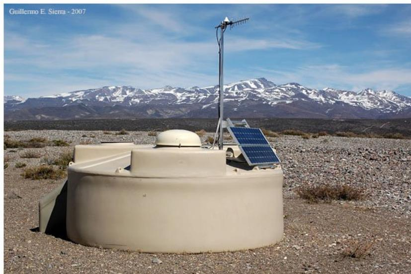
Figure 2.4: A surface detector station of the Pierre Auger Observatory [9].
