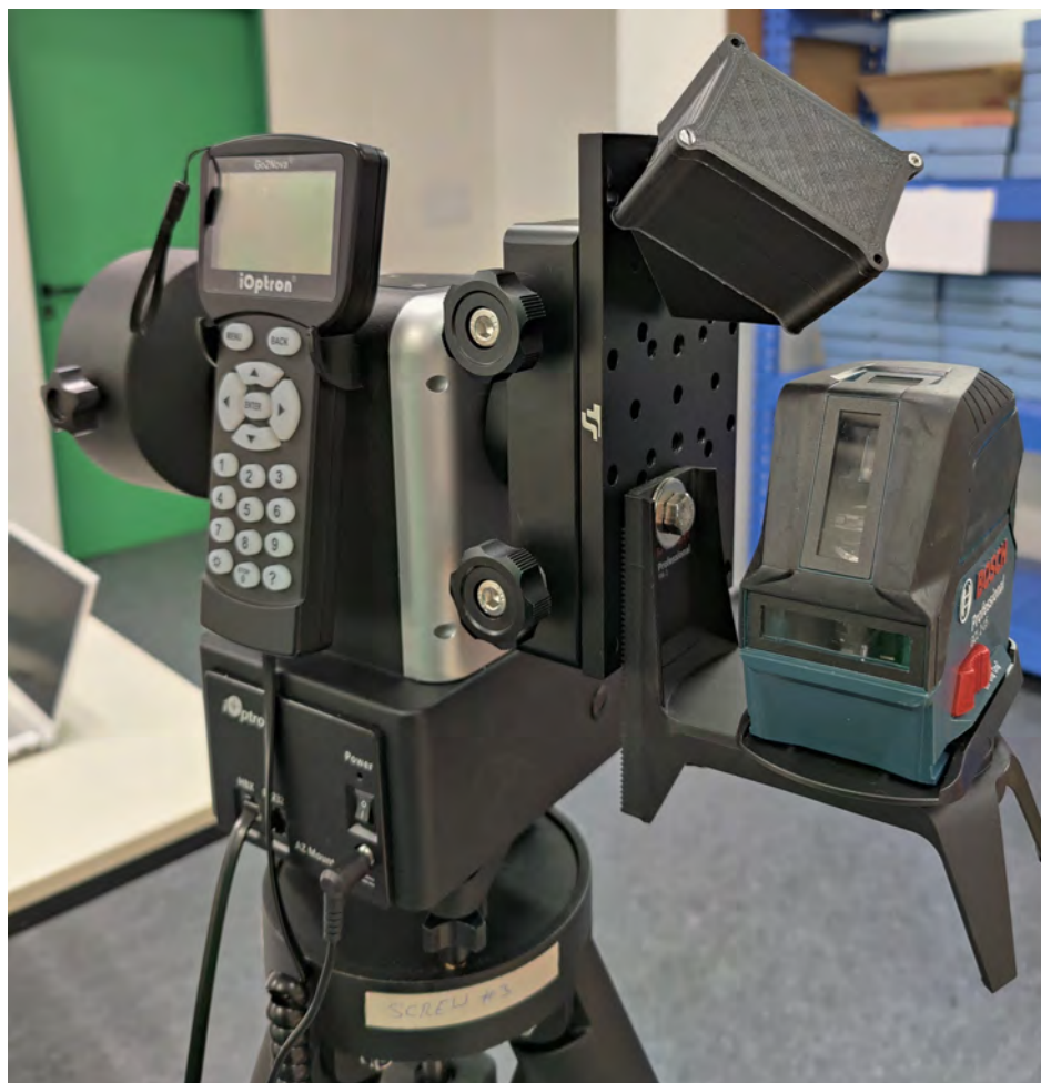
Figure 3.8: Picture of the setup with the G-sensor attached to the mount.
