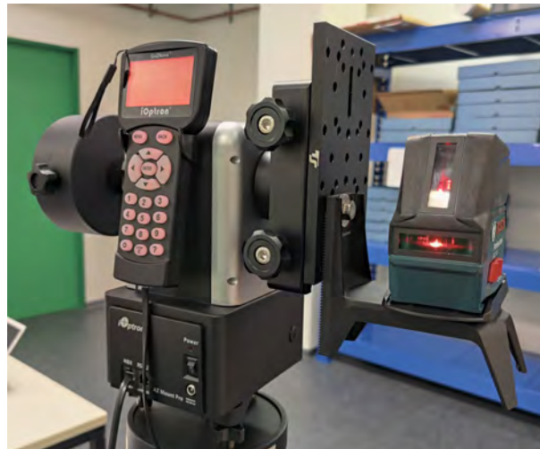
Figure 3.2: The picture shows the laser level attached to the telescope mount.
