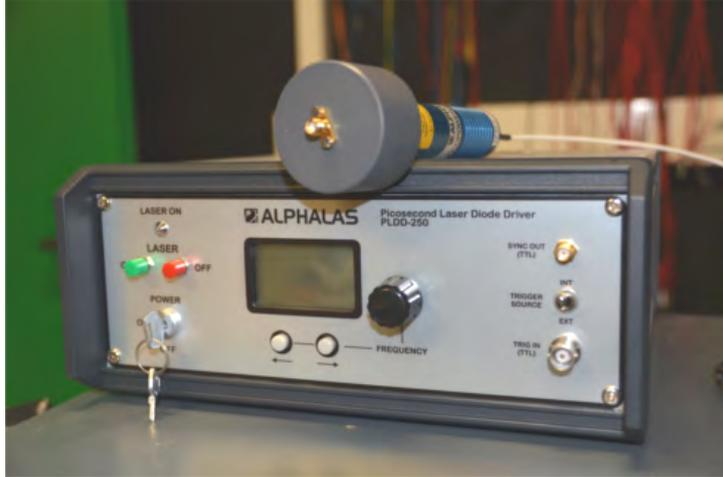
Figure A.6: Photograph of the laser diode used as light source introduced in the diffuse reflectivity measurements in chapter 4 section 2
