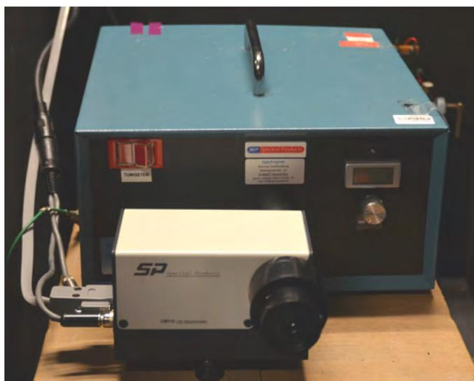
Figure A.2: Photograph of deuterium-tungsten light source used for intergrating sphere measurements
