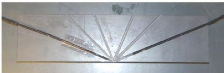
Figure 6.1: Plastic board with three grooves of the width of 1 mm optical fibres to the left and the right each, used to measure the angular distribution of light reflected off a *Tyvek* sample
