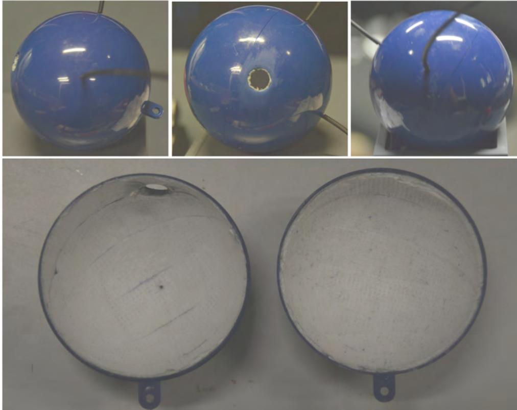
Figure 4.5: a) Photograph of the input port of the small sphere with an optical fibre stuck into it; b) Photograph of the sample port of the small sphere; c) Photograph of the exit port of the small sphere with an optical fibre stuck into it; d) Photograph of the small sphere divided in two halves; all ports are in the left hemisphere, with the central point depicting the input port, the large whole depicting the sample port and the point at the left depicting the exit port
