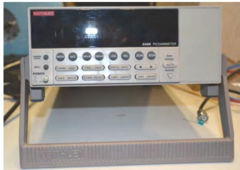
Figure A.4: Photograph of the amperemeter used for measuring the photo current
