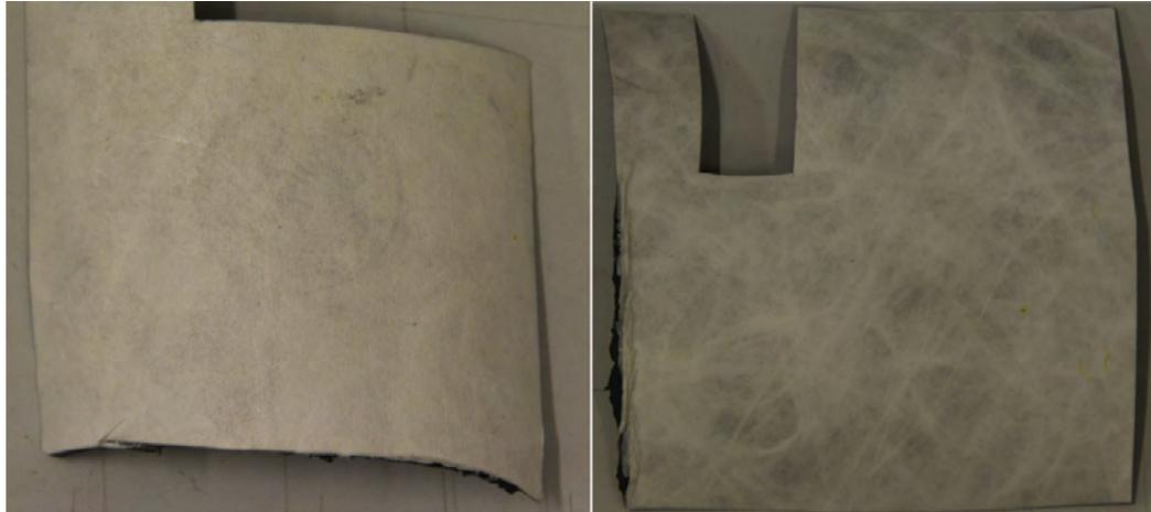
Figure 3.1: a) Sample of unused *Tyvek*; b) Sample of used *Tyvek*; structural differences are visible, especially the black "spots" in the used sample
