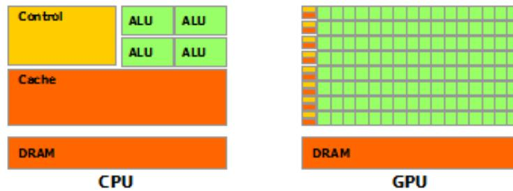
**Figure 1.4:** Schematic view of a CPU (left) and a GPU (right). Each box represents the space on the chip used for a specific function indicated by the color [10].
