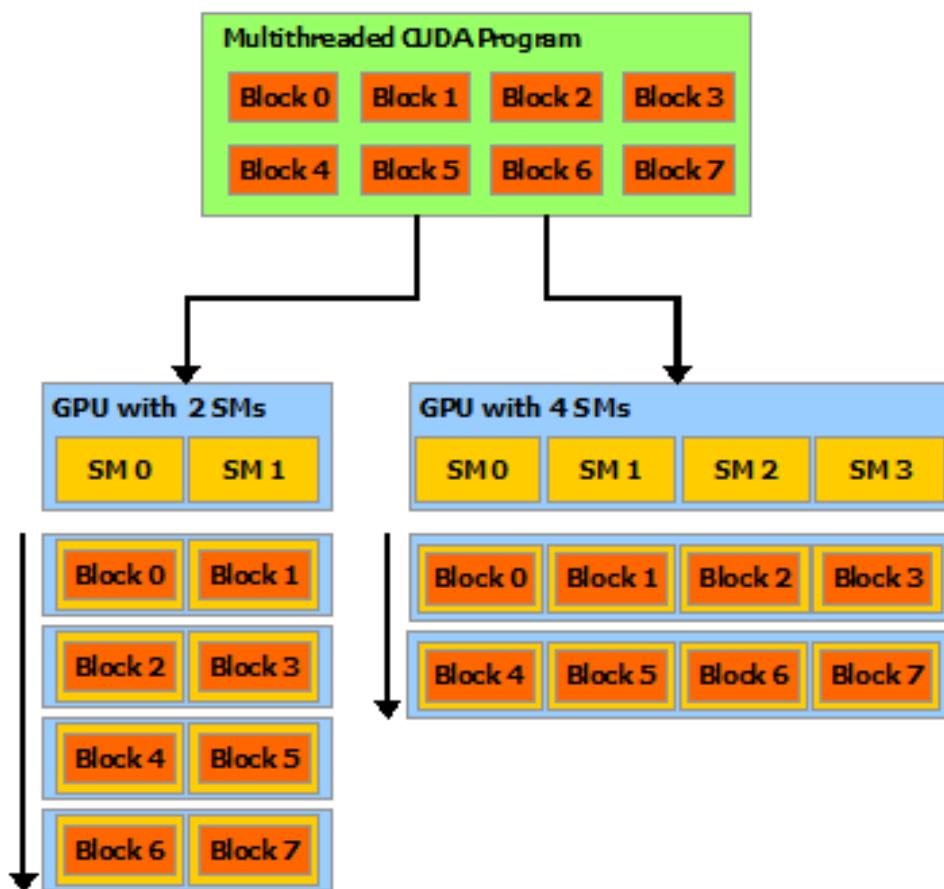
Figure 1.5: Execution of a multithreaded CUDA program on two GPUs with a different number of Streaming Multiprocessors [10].
