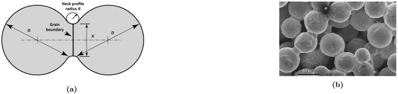
**Figure 3.3:** Schematic of a sintered particle (a). Two particles stick together at the grain boundary (sinter neck). Sinter neck formation of bronze particles in a scanning electron micrograph (b) (German, 2014).
