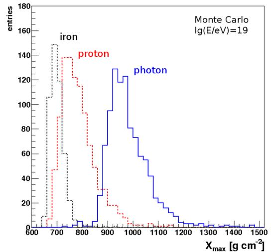
Figure 1: Discriminating observable for the Auger fluorescence detector: the depth of shower maximum,  $X_{\max}$ . Distribution of  $X_{\max}$  are shown for Monte Carlo events induced by photons (solid blue line), protons (dashed red line) and iron nuclei (dotted black line) at 10 EeV.
