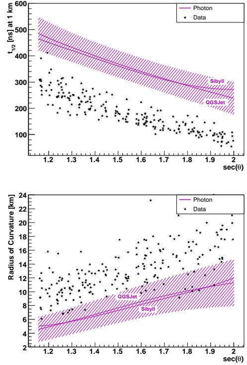
Figure 3: Discriminating observables for the Auger ground array: upper panel the signal risetime  $t_{1/2}$ , lower panel the radius of shower front curvature. The parameterization of the mean behavior for 20 EeV primary photons is plotted as a function of shower zenith angle along with a sample of real events. The deviation of the observed values from those expected for primary photons is evident. Figures from Ref. [6].
