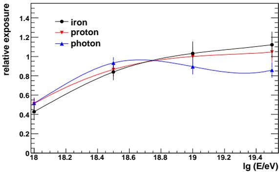
Figure 4: Relative exposure after trigger, quality cuts, and fiducial volume cuts for primary photons, protons and iron nuclei (normalized to protons at 10 EeV). Polynomial fits are superimposed to the obtained points. Figures from Ref. [8].
