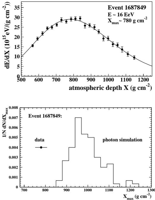
Figure 2: Upper panel: longitudinal shower profile of a typical event recorded by the Auger fluorescence detector. Lower panel: data point with statistical uncertainty along with  $X_{\max}$  distribution from photon simulations. Figures from Ref. [5].
