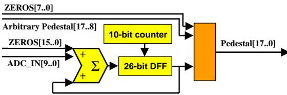
Figure 4: Pedestal selection. A native pedestal for each channel in each Front End Boards is calculated on the basis of  $2^{26}$  samples separated by intervals  $2^{10}$  time bins =  $25.6 \mu s$ . The multiplexer allows selecting a “manual” mode with a pedestal arbitrarily chosen or an “automatic” mode with pedestals optimized for each channel.
