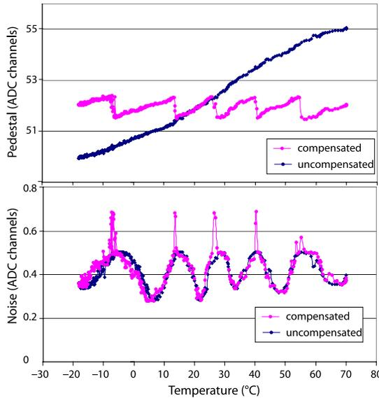
Figure 5: FADC drifts a function of temperature measured in the climate chamber. Top: The uncompensated drift range amounts to  $\approx 5$  ADC-channels. The compensated one by the sigma-delta routine stays below 1 ADC-channel. Each point in the graphs correspond to averaged pedestals over  $10^5$  measurements.
