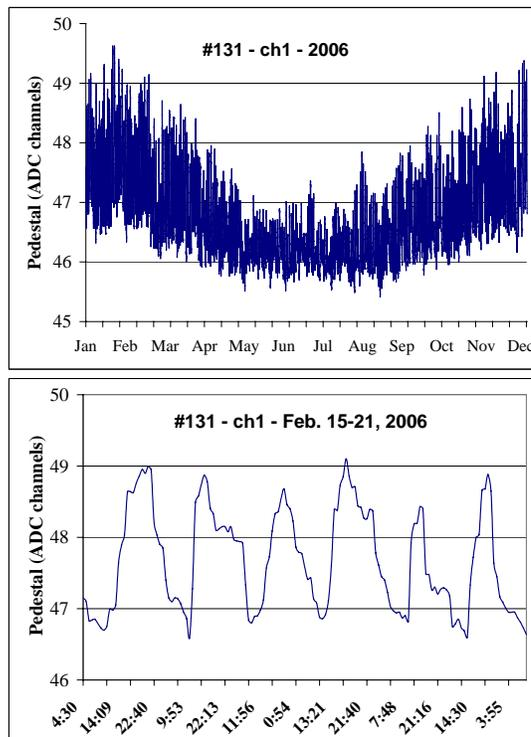
Figure 2: Dynode pedestal as a function of time (channel 1 in the Luz tank (No. 131) from Jan 1<sup>st</sup> until Dec. 31<sup>th</sup>, 2006) (top). Seasonal drift is clearly seen. Short-term variation of the pedestals for high-gain channel 1 in the Luz tank within Feb. 15<sup>th</sup>-21<sup>th</sup>, 2006 (bottom). This type of variation vs. temperature is typical for almost all Front-End-Boards in the surface detectors.
