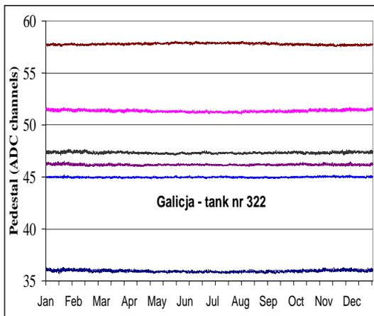
Figure 1: Pedestals as a function of time for all channels in the Galicja tank (No. 322) from Jan 1<sup>st</sup> until Dec. 31<sup>th</sup>, 2006. This tank contains the Front-End-Boards with an exceptional small variation of pedestals less than 0.67 ADC-channel in the most temperature-dependent channel.
