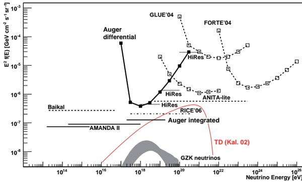
**FIGURE 5.** Limits at the 90 % C.L. for a diffuse flux of  $\nu_\tau$  assuming a 1:1:1 ratio of the 3 neutrino flavors ([24] and references therein) and predictions for a top-down model [25].
