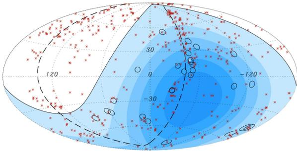
**FIGURE 7.** Aitoff projection of the celestial sphere in galactic coordinates. The positions of the AGN within  $D < 71$  Mpc (stars) and of the events with  $E > 57$  EeV (circles) are marked. The colors indicate equal exposure [8, 30].
