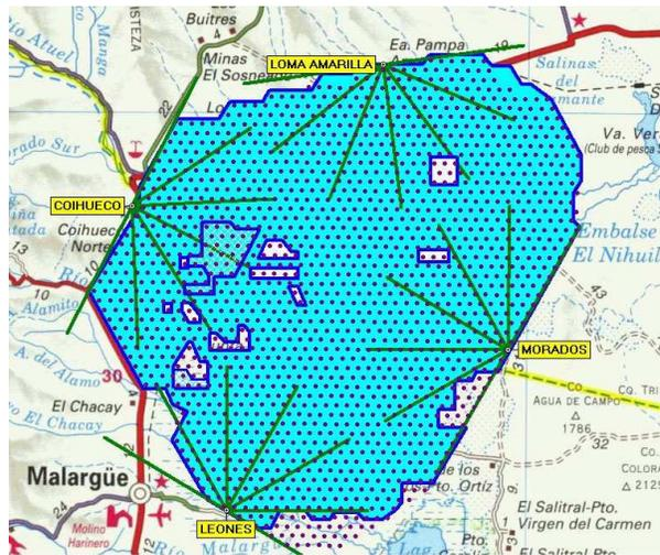
**FIGURE 1.** Layout of the southern site with the locations of the surface detector tanks indicated. Also shown are the locations of the fluorescence observation sites with the f.o.v. of their telescopes. The blue region indicates the part of the ground array currently in operation (May 2008). Furthermore, all 24 telescopes distributed over the four sites Los Leones, Coihueco, and Loma Amarilla and Los Morados are in operation.
