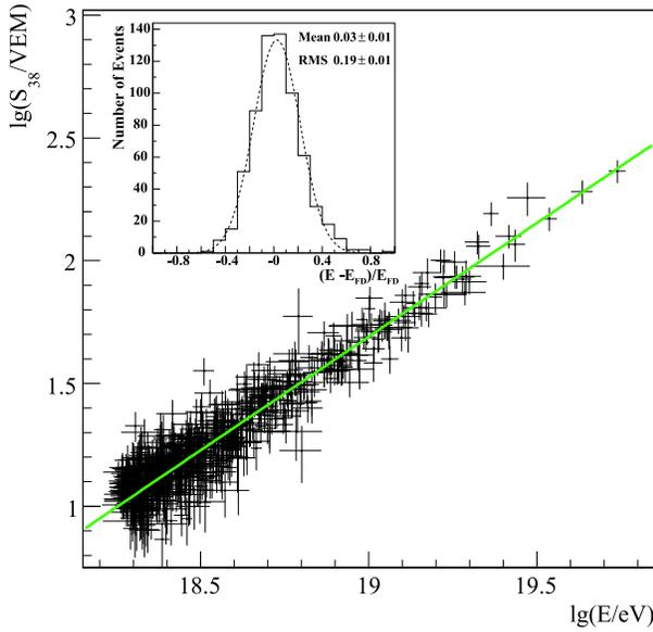
**FIGURE 2.** Correlation between  $\lg S_{38^\circ}$  and  $\lg E_{FD}$  for hybrid events. The full line is the best fit to the data. The fractional difference between the FD and SD energies is shown in the inset [7].
