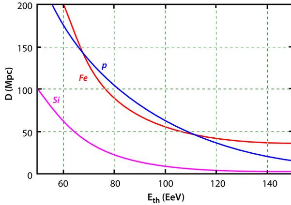
**FIGURE 8.** GZK-horizon, defined by 90 % of the observed particles originating from within the horizon scale, for p, Si, and Fe nuclei assuming an energy spectrum  $\propto E^{-2.7}$ . (Data from [4].)
