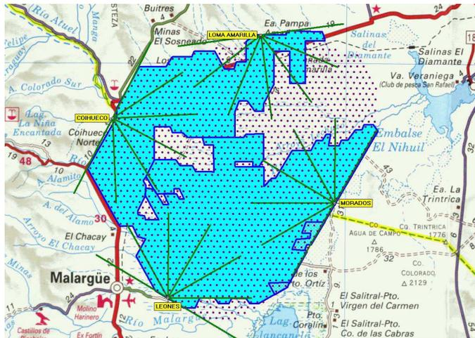
Figure 1: Layout of the southern site with the locations of the surface detector tanks indicated. Also shown are the locations of the fluorescence eyes with the f.o.v. of their telescopes. The blue region indicates the part of the ground array currently in operation (Febr. 2007). Furthermore, all 24 telescopes distributed over the four sites Los Leones, Coihueco, and Loma Amarilla and Los Morados are in operation.
