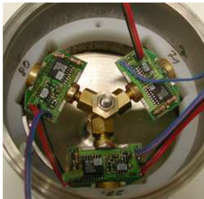
Figure 5.1: Inside view of one first generation SPATS sensor housing (without voltage converter board) used at SPATS strings A-C [Bös 06].
