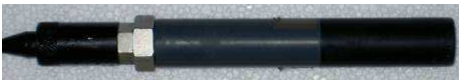
Figure 6.11: Absolutely calibrated hydrophone Sontortech SQ03. The acoustic sensitive area is the black part on the right side.
