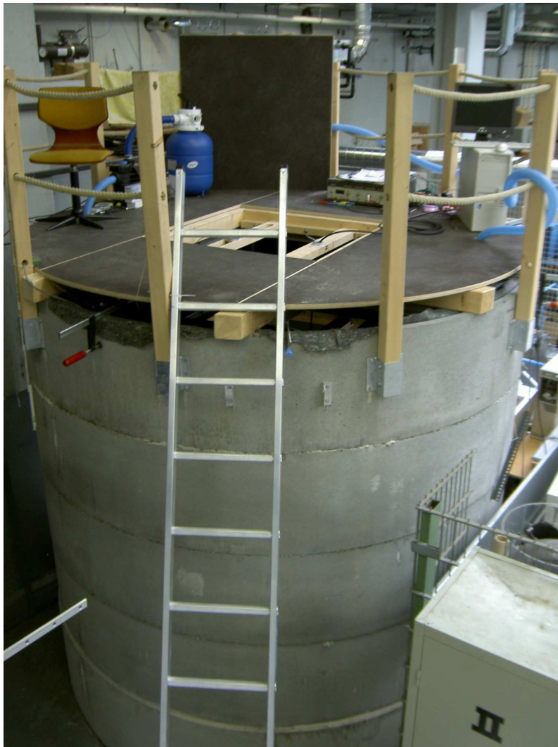
Figure 7.1: Wuppertal Water Tank Test Facility with walkable platform, installation opening and pump with sand filter (blue).
