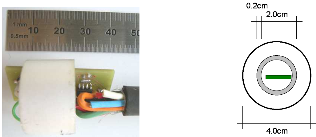
Figure 5.5: HADES sensor without PU coating (left side) and schematic drawing of a HADES sensor (bottom view). The piezo electric element (gray ring) with the amplifier board (green) are surrounded by hard PU coating (right side).
