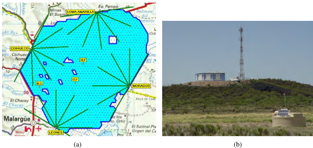
Figure 1.14.: On the left, a schematic view of the Pierre Auger Observatory in April, 2009. All surface stations (blue points) in the green area were deployed at this time. The right picture shows one surface detector station in the field with a fluorescence telescope building in the back.
