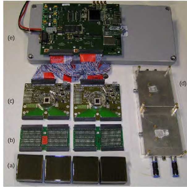
Figure 5.5 – Photograph of all components of the readout chain consisting of four MAPMTs (a), two attenuator boards (b), two n-xyter FEB modules (c), water colling plate (d), and SysCore ROC (e). The analogue signals from the MAPMT to the ADC on the front-end board are transmitted on PCB tracks and connectors without cables in between. Data from the FEB to the ROC is transmitted by twisted pair flat cables. Photograph taken from [137].
