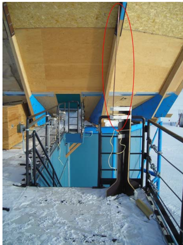
(b) The half arm dipole in z direction deployed on the front right part of the MAPO roof called "roof 2 z".
