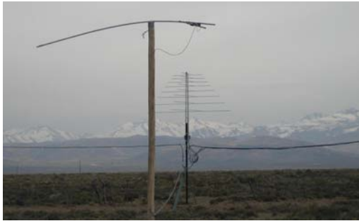
(a) The 3 m Antenna on top of a wooden pole in front of a LOPES logarithmic periodic dipole antenna.
