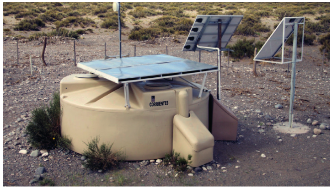
Figure 2.7: Photograph of a prototype of a surface scintillator detector station for the PAO upgrade AugerPrime [61].
