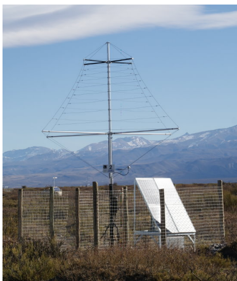
(a) AERA station: Two crossed LPDA with custom electronic [30]
