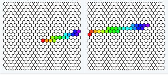
Figure 7. Light track of a hybrid event as seen by two adjacent fluorescence cameras. The zenith angle is  $\theta = 71^\circ$  and the nearest distance of the EAS to the telescopes is about 20.5 km. The different colors (grey-scalers) indicate the time progression of the pixels in the respective cameras. Other traces of the same event are shown in Figs. 6(b), 9, and 10.
