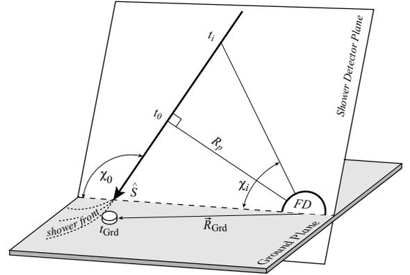
Figure 8. Illustration of the geometrical shower reconstruction from the observables of the fluorescence telescopes.
