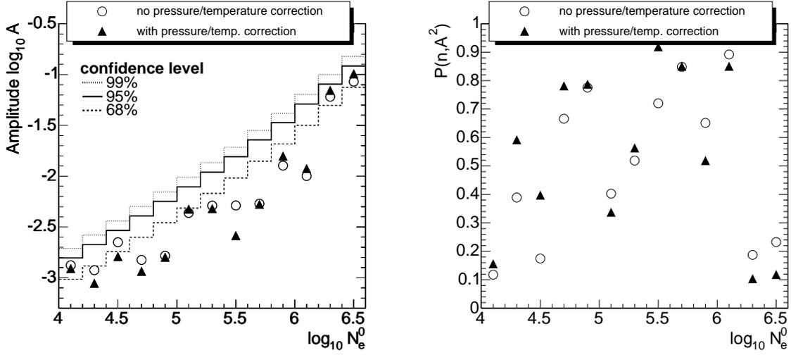
Fig. 4.— Result from the Rayleigh analysis for showers without and with correction for atmospheric ground pressure and temperature. Left-hand side: Rayleigh amplitude  $A$  vs. electron number  $\log_{10} N_e^0$ . Right-hand side: Probability  $P(n, A^2)$  that the amplitudes plotted in the left figure are fluctuations from underlying uniform distributions.
